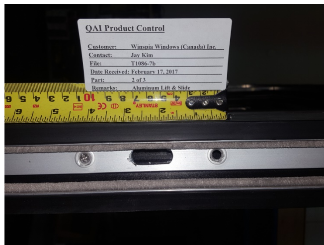
Figure 9: Top locking point of multipoint assembly, active slab.
