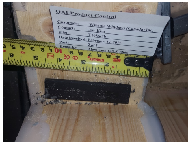
Figure 36: Shim at jamb.
