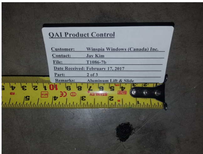
Figure 4: Fiber drain plug used in drainage holes at sill interior.
