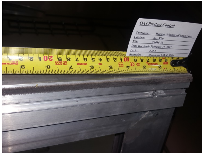
Figure 22: Modified “meeting stile cover” fastened to active slab. Pile weather-strip.
