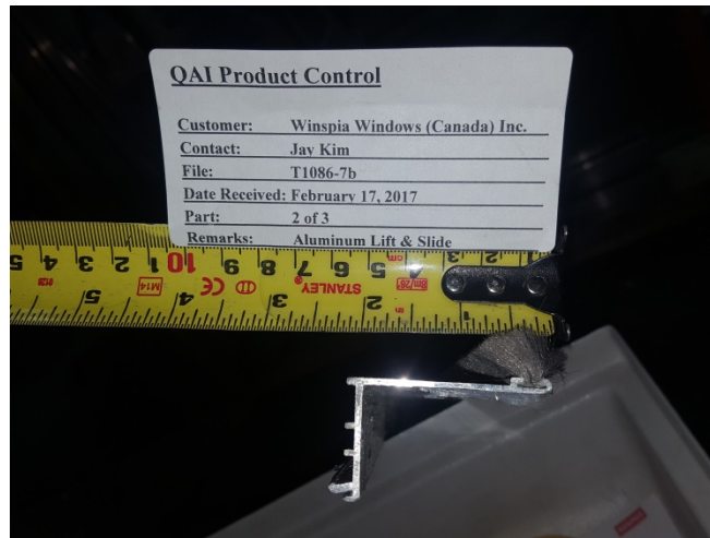
Figure 28: "Wind screen bar" profile with pile weather-strip.
