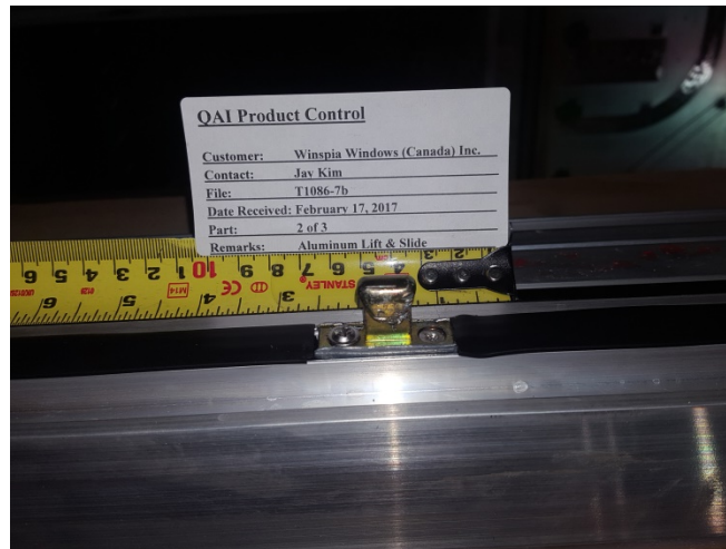
Figure 13: Keeper at locking-side jamb. Gasket on jamb around keeper.
