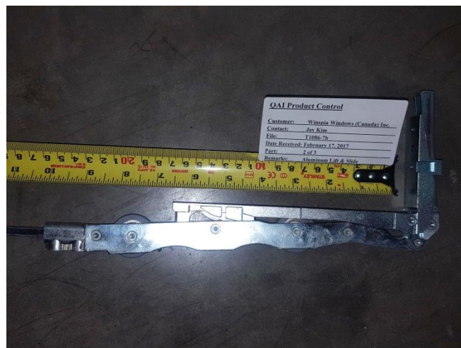
Figure 15: Rollers at bottom of active slab, locking-side corner.
