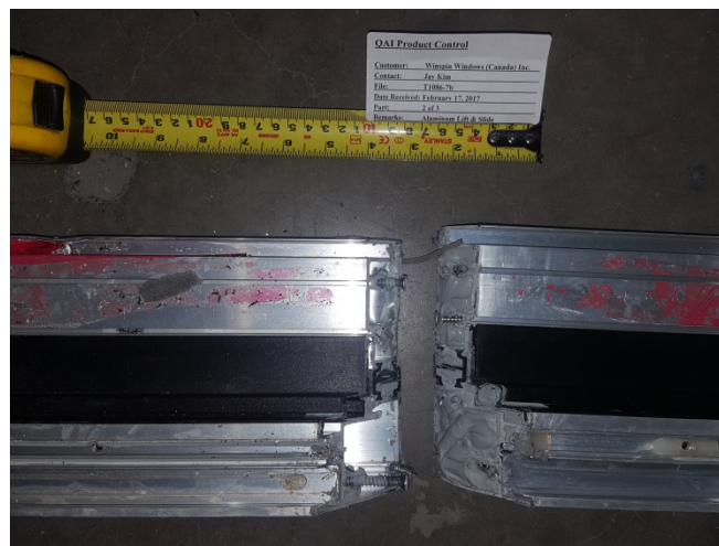
Figure 35: Fasteners at frame corner joints.
