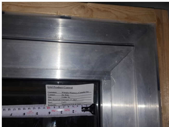
Figure 1: Corners of frame, slab, glazing bead. Silicone between buck and specimen.
