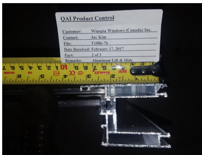
Figure 32: Slab profile consisting of "vent out" and "vent in" profiles.
