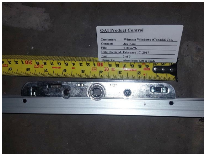
Figure 18: Gear at middle of multipoint assembly.
