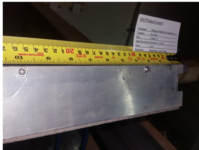
Figure 21: Modified "meeting stile cover" fastened to active slab.
