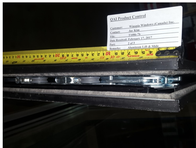
Figure 14: Rollers at bottom of active slab, locking-side corner.
