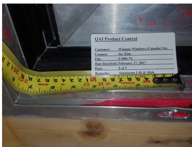
Figure 2: Drainage slot at sill exterior.
