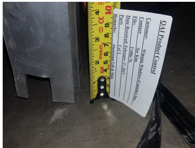
Figure 20: Slot at bottom of active slab interlock.
