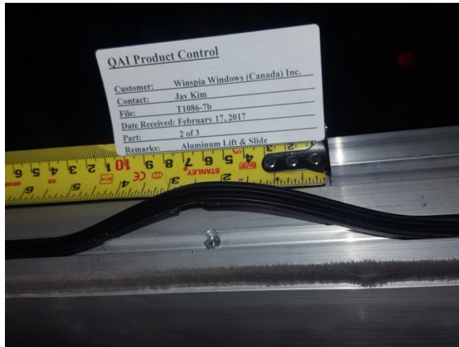
Figure 24: “Meeting stile cover” fastened to in-active slab. Weather-stripping.
