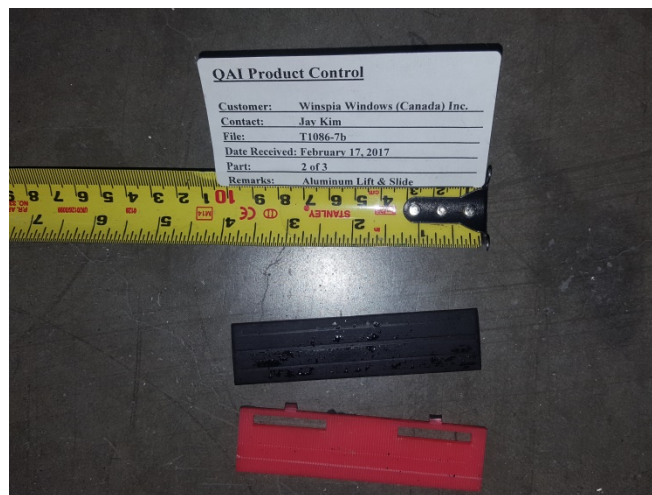
Figure 8: Setting blocks making up one setting block assembly, in-active slab.
