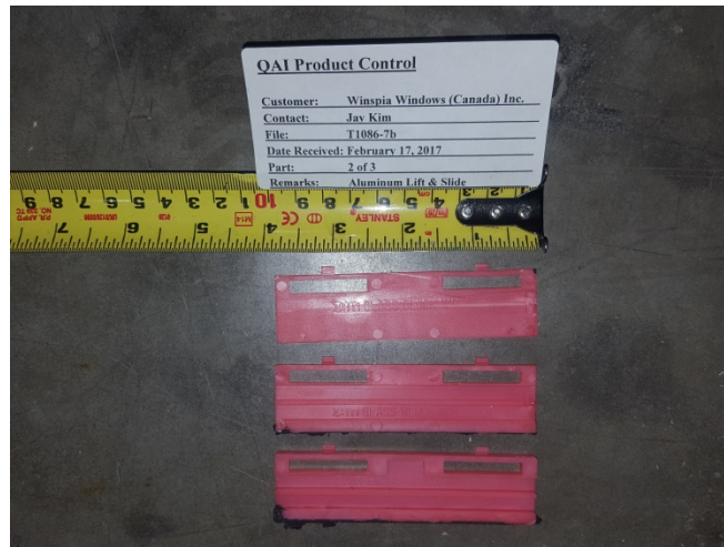
Figure 7: Setting blocks making up one setting block assembly, active slab.
