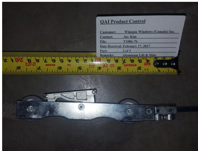
Figure 17: Rollers at bottom of active slab, interlock-side corner.
