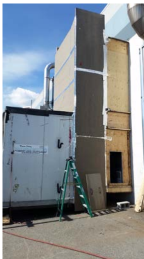
Figure 6. Test Set-up for Thermal Cycling
