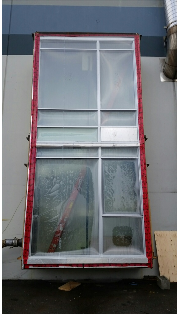
Figure 4. Completed Installation and Air Leakage Set-up
