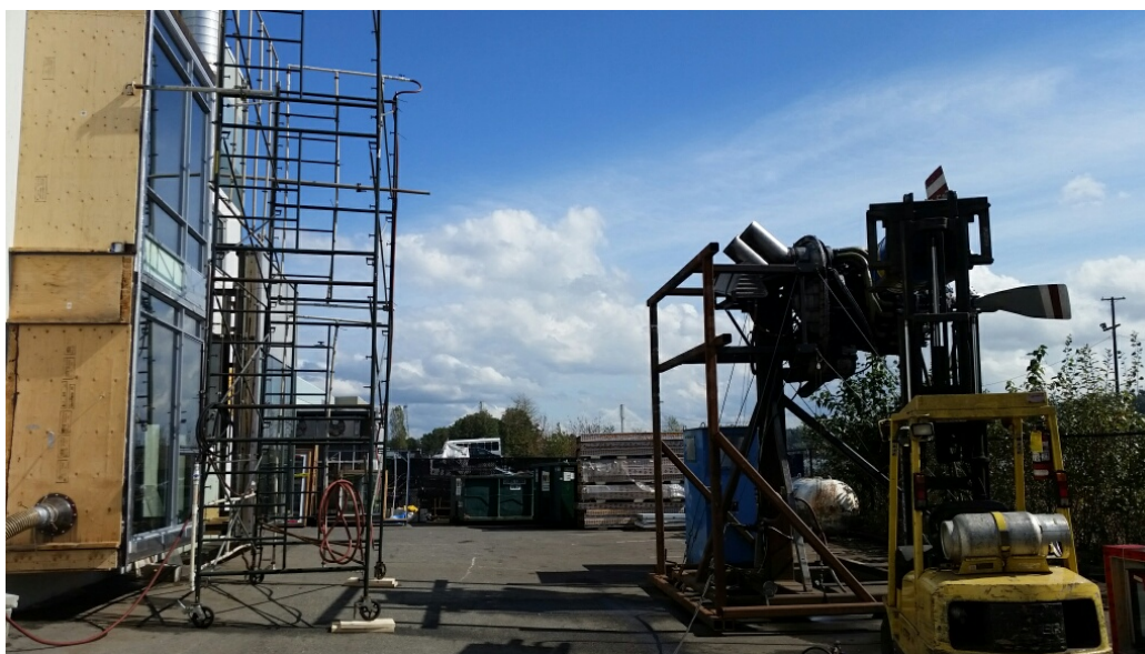
Figure 5. Test Set-up for Dynamic Water Penetration
